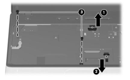
10. Lift the rear edge and sides of the top cover ① to release it. Move the top cover backward ② and place it on the base enclosure.
